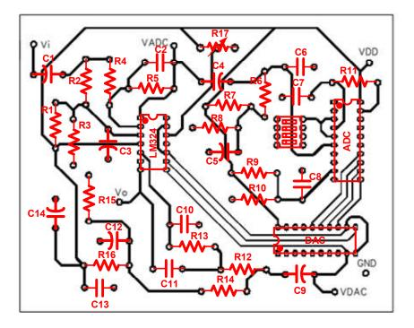
Fig. 4. PCB Layout of the AFE circuits
