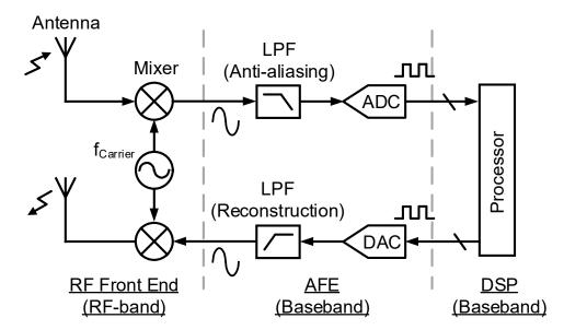
Fig. 1. The block diagram of a transceiver
