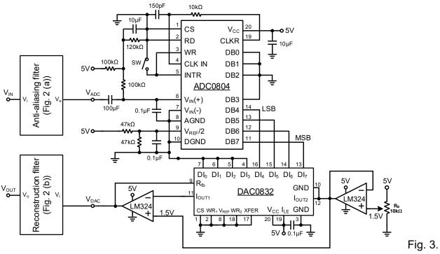
Schematics of peripheral circuits for ADC and DAC
