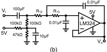
Fig. 2. Schematics of (a) the anti-aliasing filter and (b) the reconstruction filter
